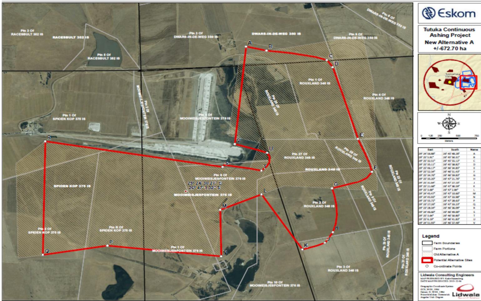
**Figure 11.3:** Alternative A - Proposed (Technical) footprint for the Tutuka Power Station Continuous Ash Disposal facility.
